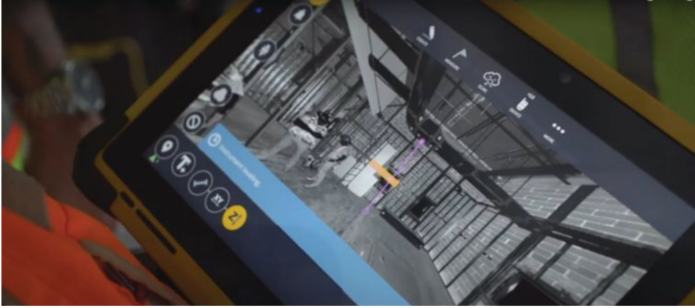
A scan of recently installed ductwork provides almost-immediate feedback on as-built conditions.
