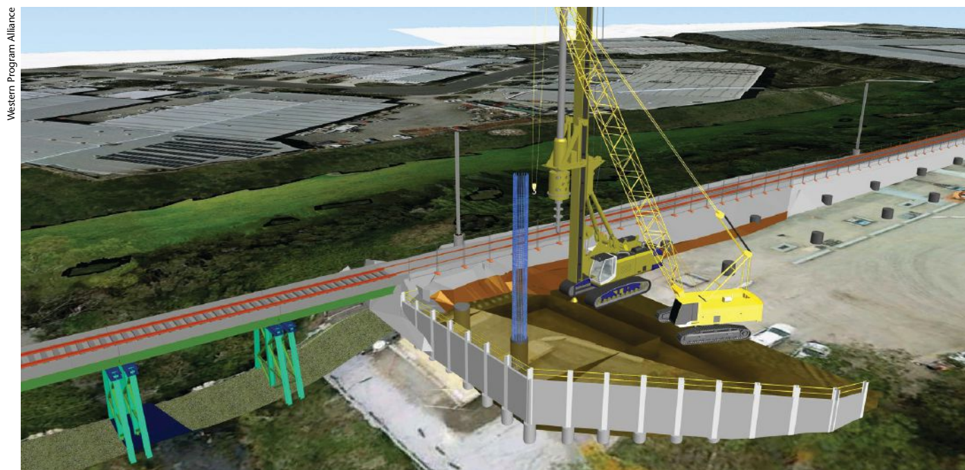
Western Program Alliance used reality capture with 4D construction modeling for a level crossing-removal project in Melbourne, Australia.
