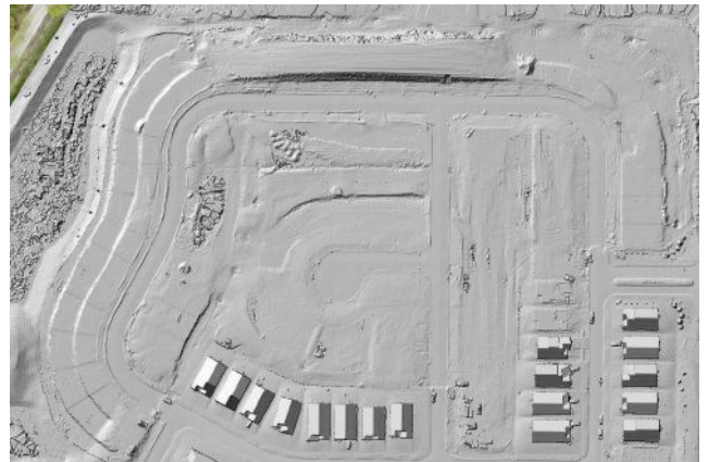
A point cloud describes highly accurate and detailed 3D mesh for earthwork volumes from drone imagery.
