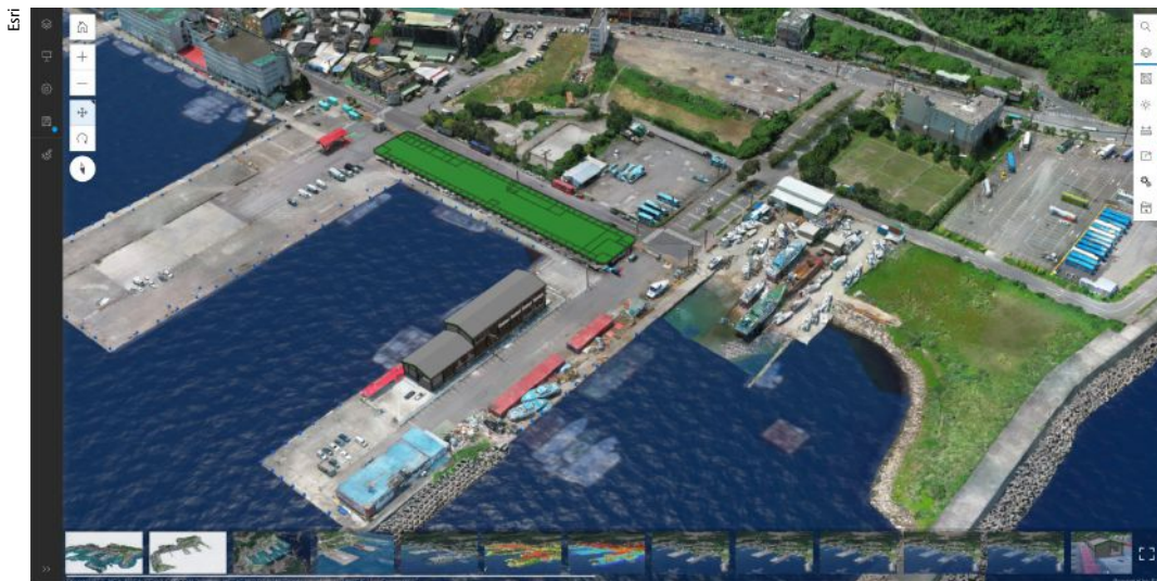
A cloud-hosted digital twin of a Taiwanese port incorporates GIS data, drone-captured 3D mesh and BIM models. It's used here to simulate the effects of sea-level rise.
